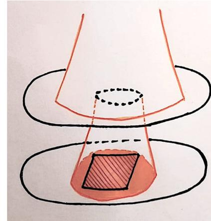
$$c = \frac{\text{hits inside TES}}{\text{total hits on the MiC plate}}$$
