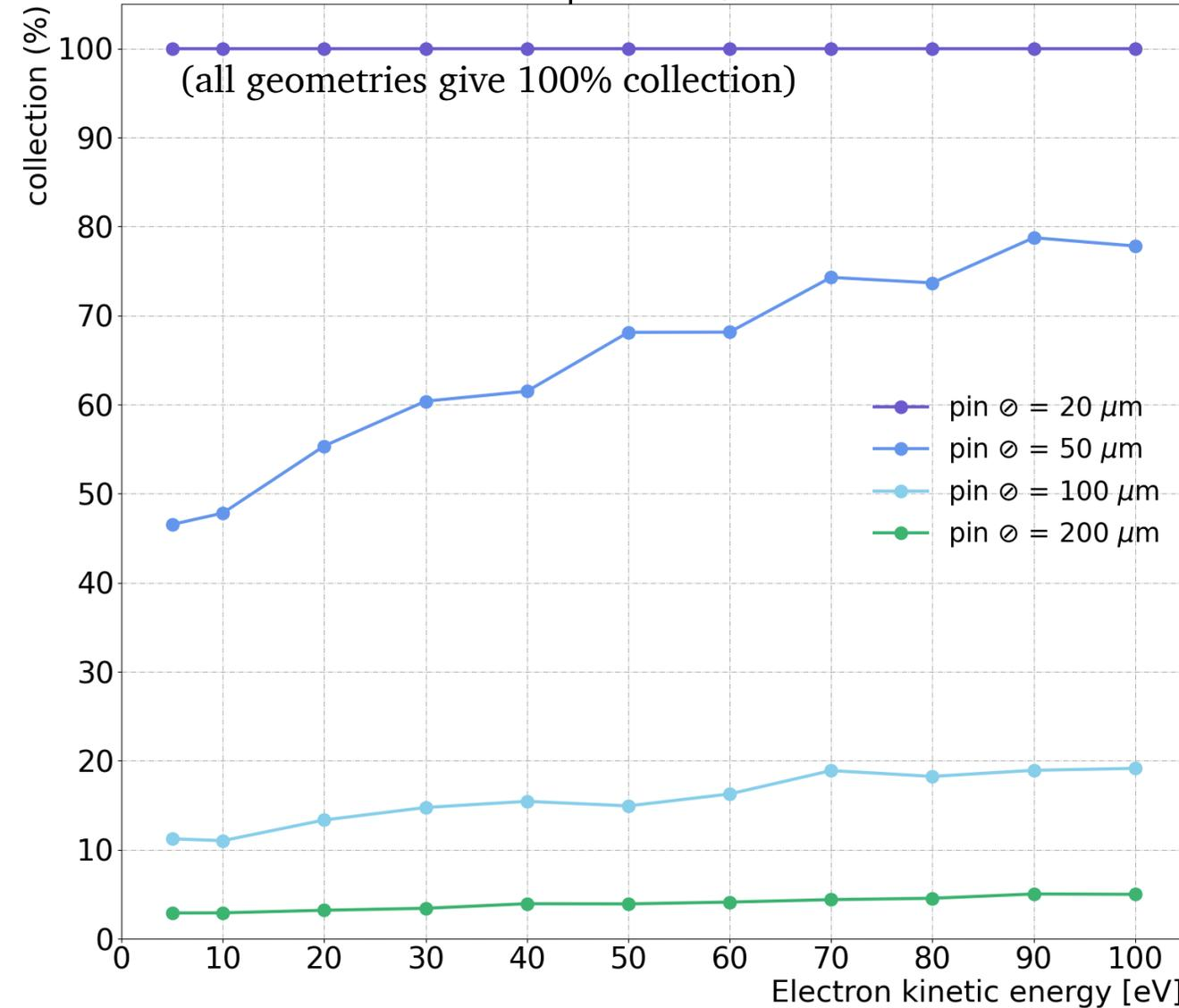
$$c = \frac{\text{hits inside TES}}{\text{total hits on the MiC plate}}$$
